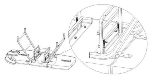
Then connect the tray bracket to the connecting tube and tighten it with screws, as shown in the photo below.
